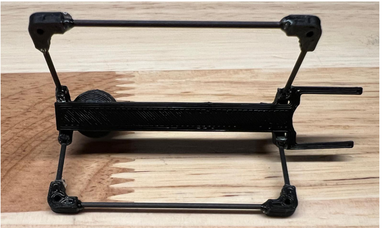
The frame is constructed using 3D printed ABS plastic parts and carbon fiber rods
