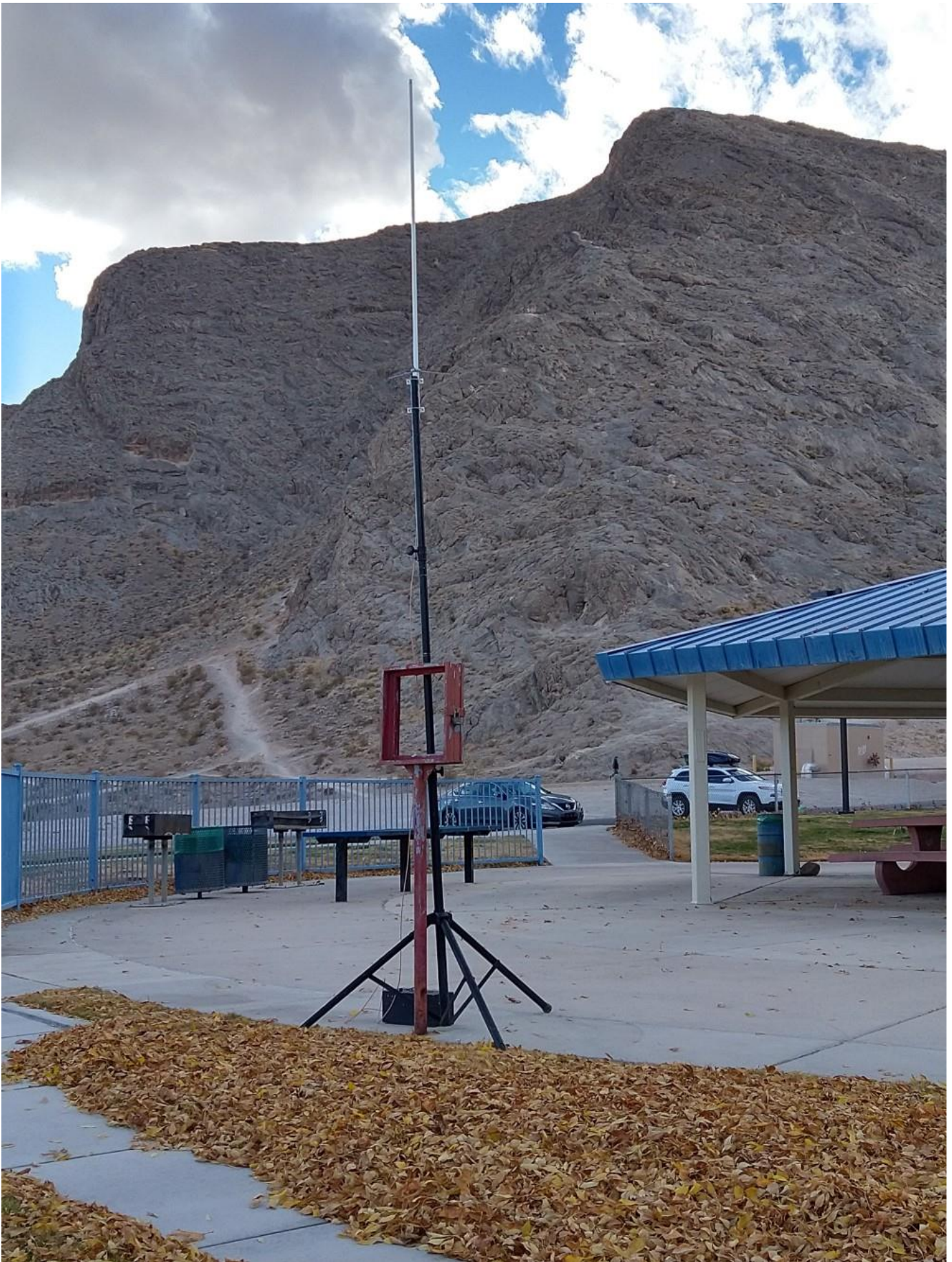
Due to the strong winds the antenna's tripod had to be tied to a sign post.
