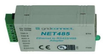
The Grid Connect NET485 converts the RS-485 status data from the EPever's charge controller into a TCP/IP transport layer, which is then passed over the LVMesh Network.
